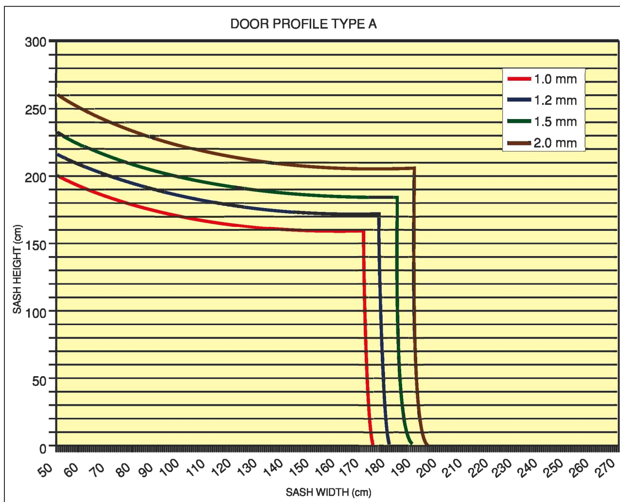
SASH HEIGHT LIMITS DEPENDING ON THE WALL THICKNESS OF REINFORCEMENT STEEL
