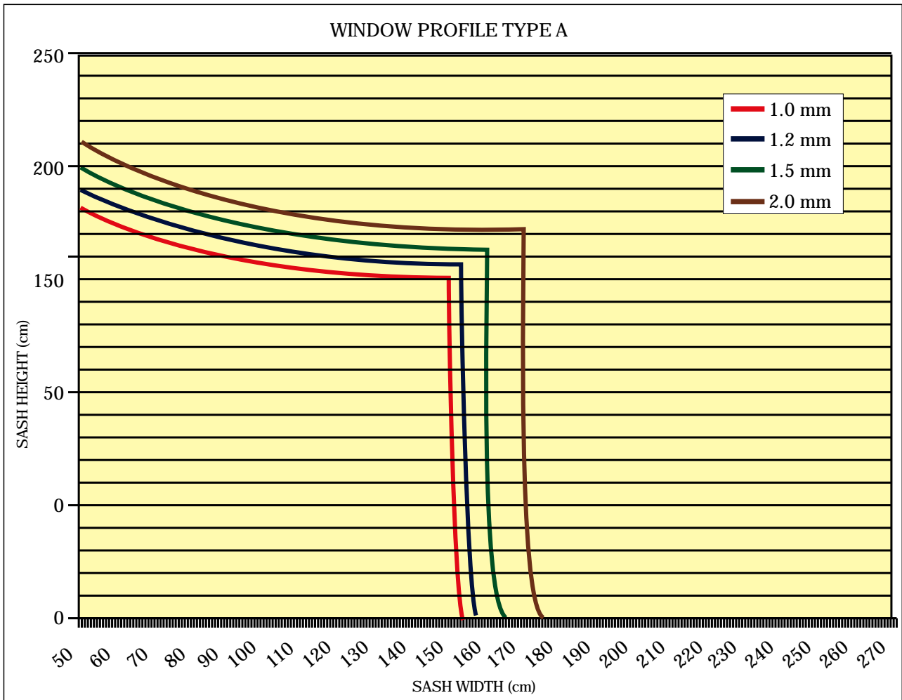
SASH HEIGHT LIMITS DEPENDING ON THE WALLTHICKNESS OF REINFORCEMENT STEEL
